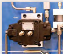
Unloader Valve on 950-HT1
